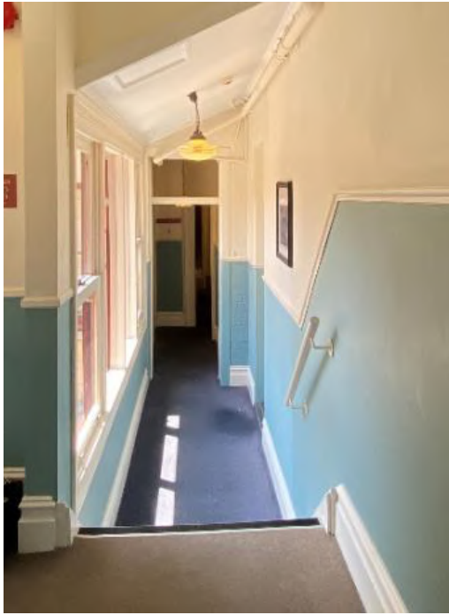
Figure 157: Hallway 2.07, looking east towards the front of the building, was formed in the 1980s by enclosing an open verandah that originally provided access from the front (1887) wing of the building to the rooms of the rear (1913) addition and the rear stair. Most of the fabric is modern, but some elements are original. Source: TKD Architects 2020.
