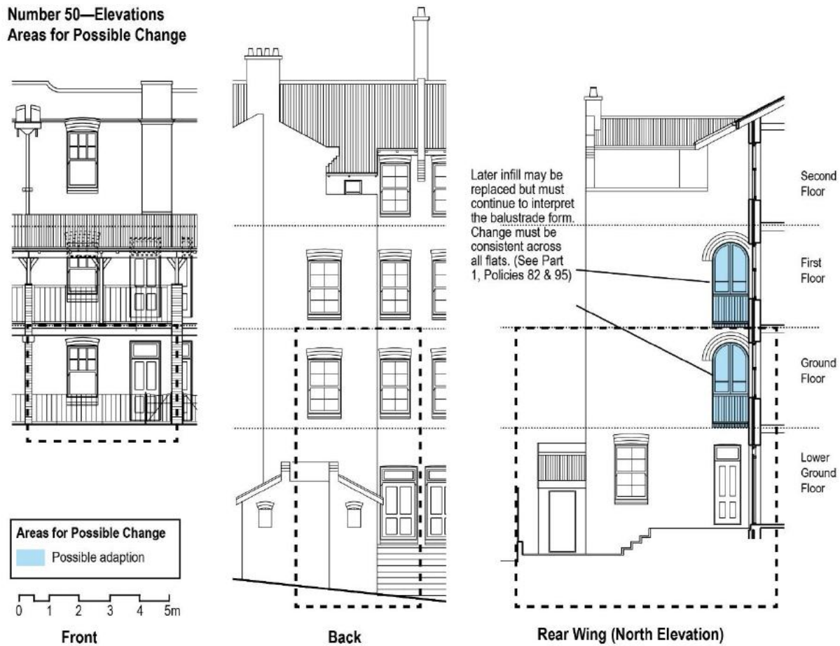
Figure 5.49 Plans showing areas for possible change—Flat 50 / 46–56 Gloucester Street. (Source: LAHC, with GML overlay 2016)
