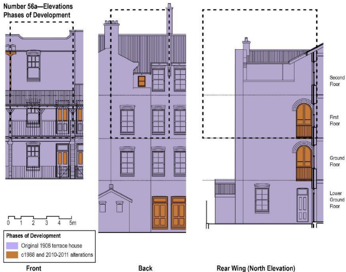
Figure 14.5 Elevations showing phases of development—Flat 56A / 46–56 Gloucester Street. (Source: LAHC, with GML overlay 2016)
