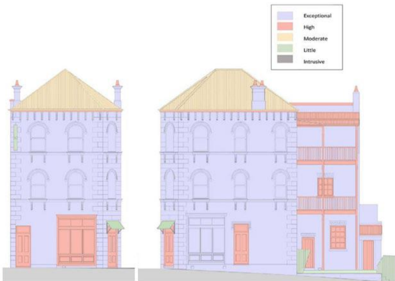
Figure 180: West elevation (left) and south elevation (right) showing grading of significant elements. (Source: 2015 CMP pp163-164, with PMNSW overlay 2024)
